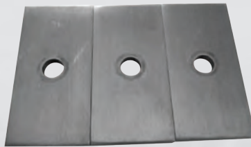
Following ASTM D2570 corrosion testing, cast iron plates show no signs of corrosion.
