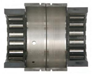
The main bearings showed only trace to light wear despite 534 hours of rigorous use, most at the Evinrude E-TEC engine's factory-lean oil setting. They earned a nearly perfect 9.95 merit rating for deposits.
