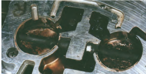
Picture J - Carburetor plates before P.i. treatment
