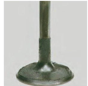
Picture E - Intake valve after P.i. treatment
