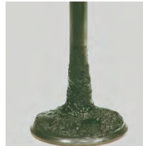
Picture D - Intake valve before P.i. treatment
