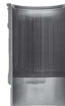
Severely Scuffed Liner
